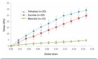
Figure 2: Mean maximum stress-strain curves for excipients processed using identical conditions; freeze-drying runs were carried out in triplicate for trehalose and sucrose (n=10 per run), single run for mannitol
